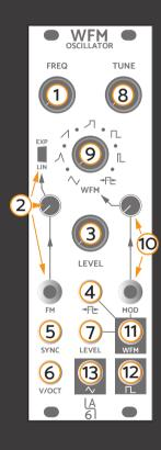
TUNE knob provides fine tuning of the output frequency.
